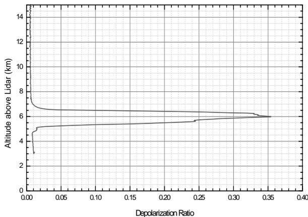
Fig. 5. Volume depolarization ratio profile through a thin cirrus layer acquired during atmospheric testing..
