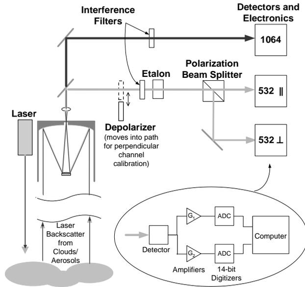
Fig. 1. Functional block diagram of CALIOP.
