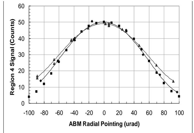
Fig. 6. Beam profiles from boresight x- and y-scans (lines) compared with modeled estimate (symbols) assuming Gaussian beam of 100  $\mu\text{rad}$  FWHM.
