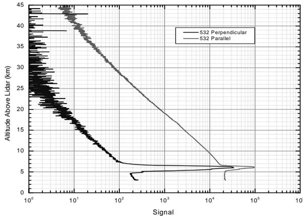
Fig. 4. 532 nm profiles (parallel, right, and perpendicular, left) acquired during atmospheric testing.
