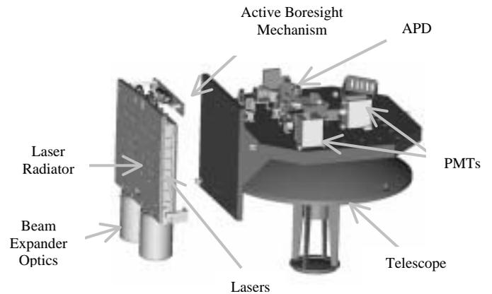
Fig. 2. Expanded 3-D rendering of the CALIOP instrument.
