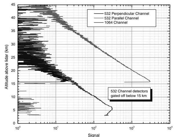
Fig. 3. Clear-air atmospheric test profiles.
