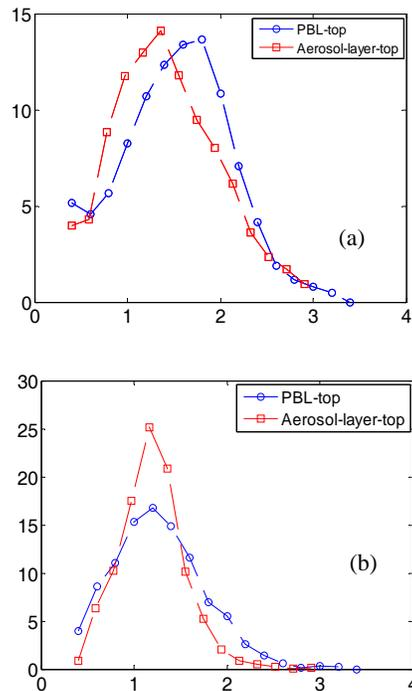
Figure 5. Histogram distribution of PBL-top and aerosol-layer-top from the CALIOP/CALIPSO data in the US continent. (a) Summer, (b) Winter.
