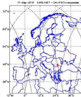
Figure 1. Bucharest's lidar station (red square) and CALIPSO ascending and descending orbits over passing Bucharest (cross lines), on 17 September 2010.
