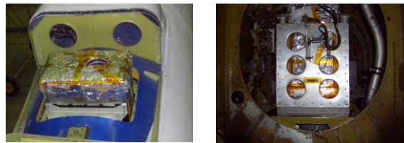
Fig. 2. MAL1 (left) and MAL2 (right) installed on M-55.
