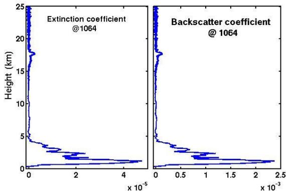
Figure 5. A vertical profile of averaged backscatter and extinction coefficient of aerosols at 1064 between 11 and 11:30.
