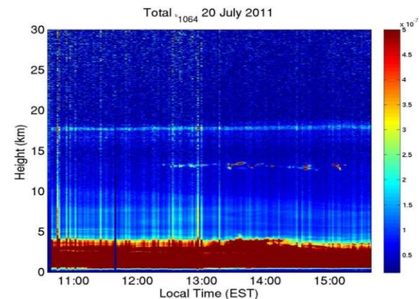
Figure 3. Backscatter coefficient of aerosol at 1064 nm. Vertical resolution is 7.5m.
