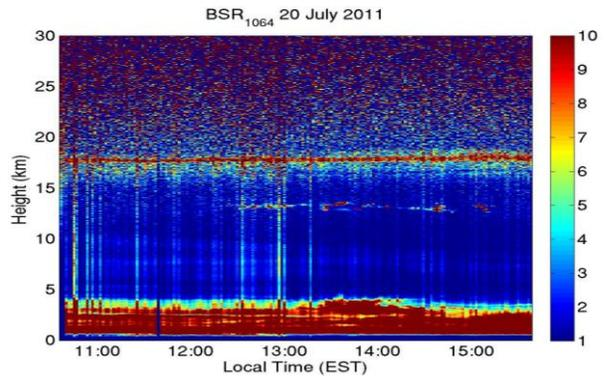
Figure 6. Backscatter ratio (BSR) at 1064 nm. A  $BSR > 3.5$  in the stratosphere is used to identify stratospheric aerosol layers.
