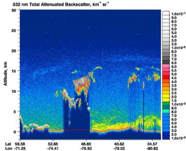
Figure 4. CALIPSO-images of total attenuated backscatter coefficient at a distance of 338 km from the Hampton observatory on 21 July
