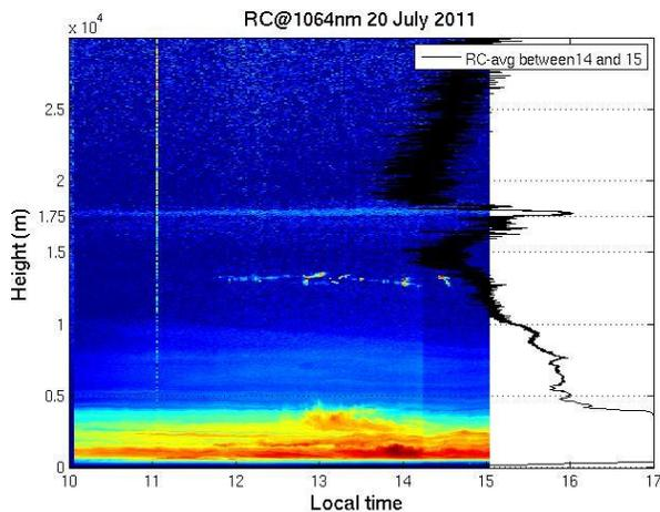
Figure 1. The range-corrected elastic backscatter signal measured on 20 July 2011 between 10:38 and 15:00 local time. The black line is the average of range-corrected signal between 14:00 and 15:00.
