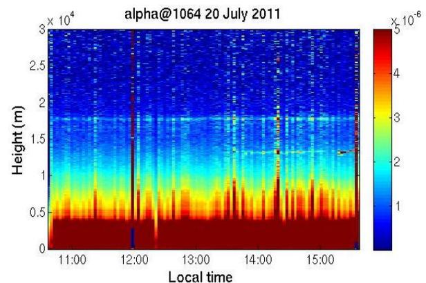
Figure 2. Evolution of extinction coefficient profiles at 1064 ( $a_{1064}$ ) using the Klett method.
