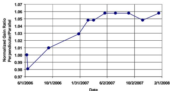
Figure 4 Polarization Gain Ratio - June 2006 to February 2008
