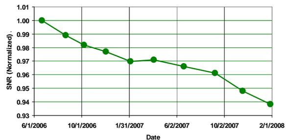
Figure 2 532 parallel channel SNR at night - June 2006 to February 2008
