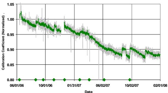
Figure 3 532 Channel Night Calibration Coefficient - June 2006 to February 2008. Diamonds across the bottom indicate the times that boresight alignments were done.
