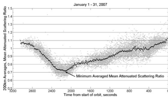
Figure 7 532 channel daytime scattering ratio as a function of time after the start of the orbit segment—January 2007
