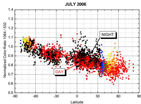
Figure 8 Color ratio (1064/532) for raw signals as a function of latitude in July. In July there is only a small difference between day (red) and night (black).
