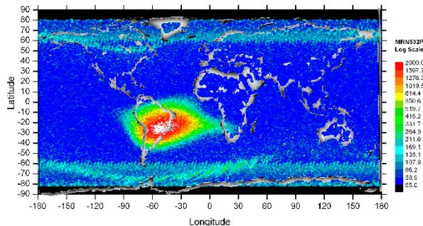
Figure 10 Geographic distribution of PMT dark noise for 16 days in April 2007 (covering all possible orbit tracks). The increased noise in the SAA can be seen clearly, along with smaller noise increases in belts around the two poles. The lighter colored horizontal bands near  $\pm 65^\circ$  latitude are from scattered sunlight.
