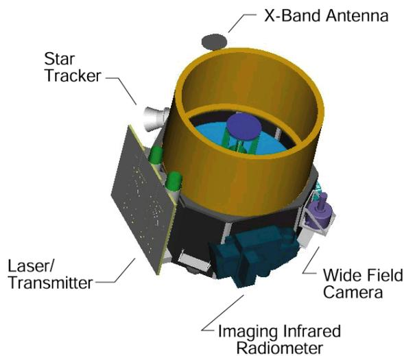
Figure 1. Schematic drawing of the CALIPSO satellite instrumentation
