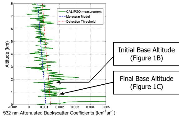
Figure 2: profile data averaged to a horizontal resolution of 20-km, taken from Figure 1(a) at  $\sim 41.3^\circ$  N (red arrow); as seen in Figure 1(b), an aerosol layer is detected between  $\sim 2.5$ -km and  $\sim 1.9$ -km, where the backscatter coefficients rise continuously above the detection threshold.
