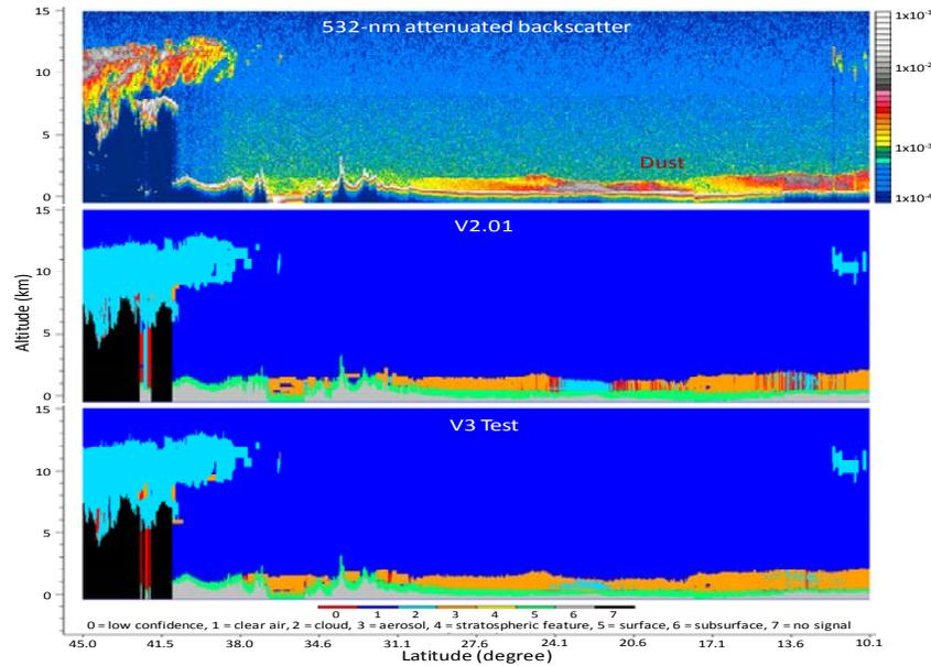
Figure 2. 532-nm attenuated backscatter (upper) and vertical feature mask (VFM) from the V2.01 data products (middle) and a V3 test data (bottom). The measurement was made by CALIPSO on Jan.1, 2007 during a nighttime orbit passing over Africa. In VFM (middle and lower panels), aerosol layers are color coded in orange, clouds in light blue, and the areas in red are mostly features with  $|\text{CAD}| < 20$  and small number of invalid features ( $< 0.01\%$ ).
