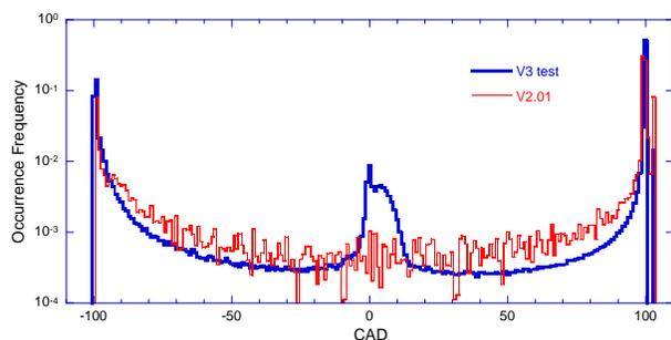
Figure 3. Distributions of occurrence frequency as a function of CAD derived from four months of the V2.01 production data using the 3D CAD algorithm and the V3 test data using the 5D algorithm. The bump between -10 and 20 in the V3 test curve, accounting for ~6% of the total features, corresponds mostly to outlier features whose physical/optical properties are not correctly derived.
