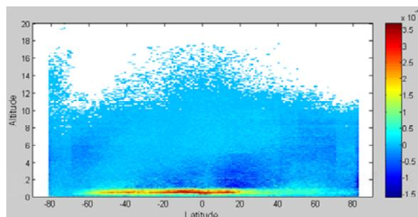
Figure 4. Vertical-latitude distribution of differential aerosol occurrence frequencies of the 5 km V3 test data and V2.01 production data (V3-V2.01). The vertical axis is the mid-layer altitude.
