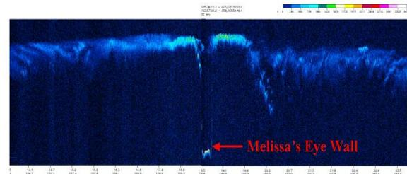
Fig 2. Distance – height lidar backscatter image of hurricane Melissa. The eye of the hurricane is also shown
