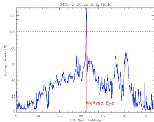
Fig 5. The isotropic albedo over hurricane Melissa showing the spike caused by reflection from near the eye wall.
