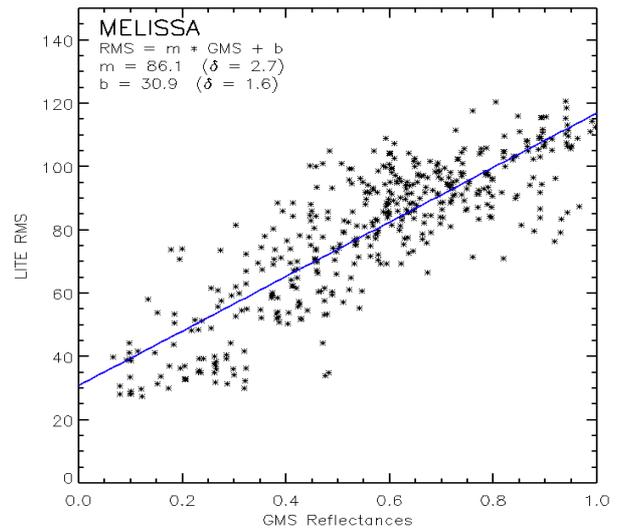
Fig 4. A plot of the GMS reflectance values measured along the orbit against the RMS noise counts.
