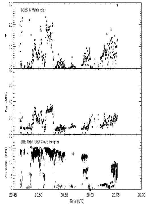
Fig. 7. The optical depth, effective radius and cloud altitude along part of the LITE orbit 80 in a tropical region from GOES satellite imagery.
