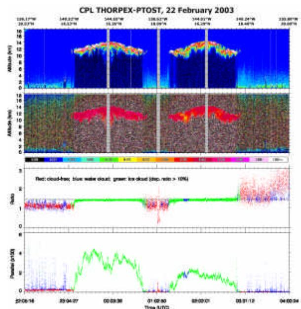
Fig.2 Attenuated backscatter at 532 nm (upper panel), depolarization ratio at 1064 nm along with color bar (second panel from top), perpendicular-to-parallel component ratio (third panel from top), and parallel component (lower panel) of background signal (mostly scattered solar radiation), observed on 22 February 2003 by CPL over the Pacific Ocean.
