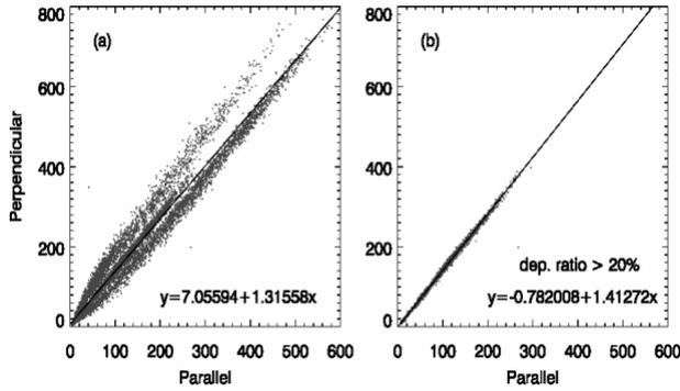
Fig.3 Scatterplots of background signals of perpendicular versus parallel components for (a) all cases and (b) for the ice-cloud only cases with linearly fitted line, for the flight of 19 February 2003.
