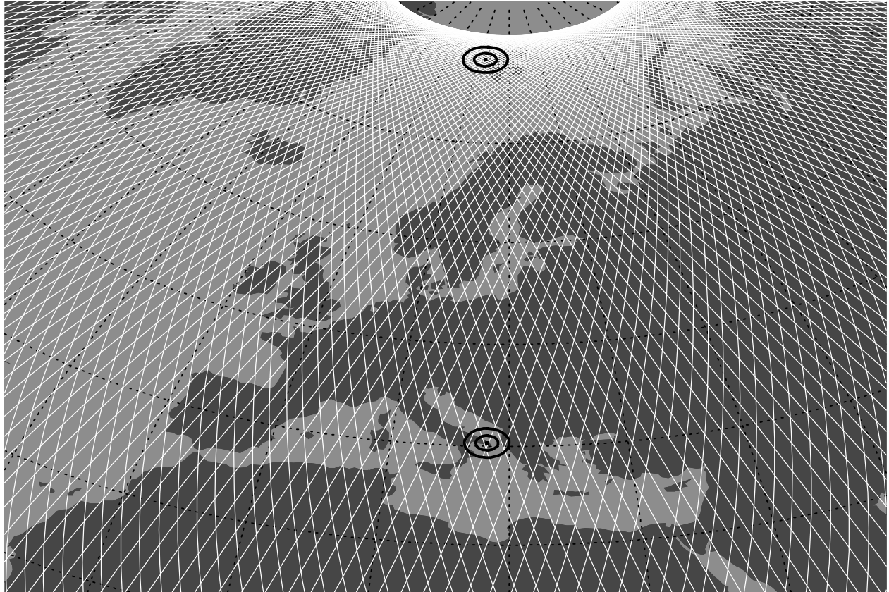
Fig. 2. CALIPSO 16-day repeating orbit ground tracks with circles around sites indicating 80 and 160 km distances.
