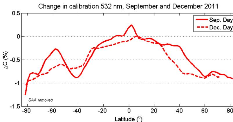
**Figure 4.** Global daytime changes in nighttime 532 nm calibration coefficients with the South Atlantic Anomaly removed.
