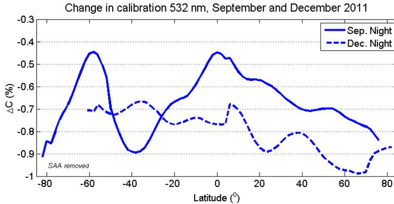
**Figure 3.** Global nighttime changes in nighttime 532 nm calibration coefficients with the South Atlantic Anomaly removed.
